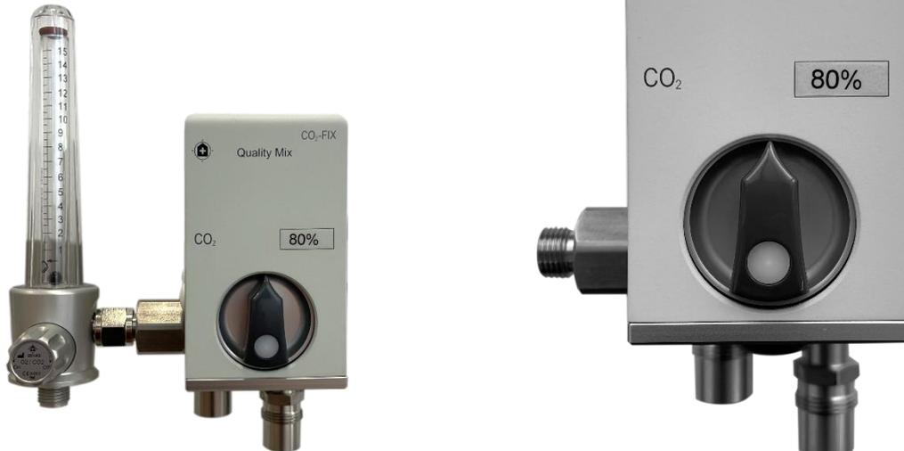
Our CO<sub>2</sub> blender for laboratory applications. The blender provides a fixed mixing ratio of carbon dioxide and oxygen that is individually adjusted according to customer requirements. The withdrawal quantity can be fine-tuned at any time with the connected flowmeter and the ratio between oxygen and carbon dioxide remains reliably constant.
